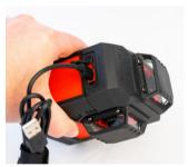
NOTE: Any standard USB A Charger or supply with 5V and 2A output can be used to charge this battery. Charger is not supplied.
