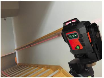
Unit featured is 360R in manual mode. Also pictured is an optional iet68 elevating tripod and optional GD12 grade dial plate; a camera style tripod with pan and tilt will provide a similar result.
